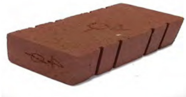
Figure 2. Sustainable red mud brick (228 mm x 108 mm x 80 mm)
