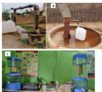
Prototype tested at Chhattisgarh (Two 10 litre tanks, 450 g adsorbent bed)
